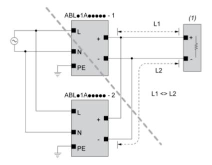
(1) : Load ABLx1Axxxxx-1 = ABLx1Axxxxx-2 max 2 x ABLx1Axxxxx L1 = L2  $\Delta V$  max 25 mV  $I_{Load} < 90\% 2 x I_{nom}$
